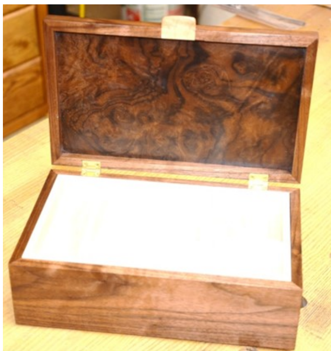
WALNUT JEWELRY BOX- SMALL MITERED BOX WITH THE GRAIN MATCHED. BILL VENEERED WALNUT BURL TO THE TOP AND USED MAPLE FOR THE SIDE TRAYS. THE FINISH IS A SPRAY LACQUER.
